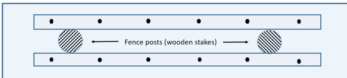
birds eye view of the seat attached to the top pf the side support panels with evenly spaced coach screws
